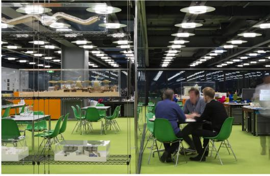
The chosen bright semi-transparent crystalline fitting is softened by a bespoke trimless 750mm white dish, and appears two ways – suspended, or surface mounted set within a perforated metal ceiling plate. These are mounted on a network of 3-circuit track, simplifying installation and controls, and adding the flexibility to add and move lighting while keeping the ceiling clean and orderly.
